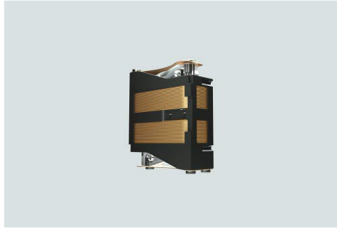
Fig. 1. The L5 actuator by Lofelt GmbH consists of a voice coil in plastic casing. A permanent magnet in the middle reacts to the magnetic field caused by the current flowing through the coil wire. Sine wave signals produce periodic upwards and downwards movements of the magnet (referring to the directions in the image). Placing the flat 17.0 \times 20.5 mm case surface against the body results in vibration parallel to the skin [1].
