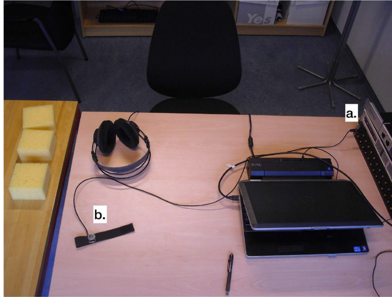
Fig. 2. Experimental setup. A PC running the experiment connects to the audio-tactile hardware system via USB. A shielded audio cable carries the pure tone signals from the amplifier output (a) to the L5 input on the wristband prototype (b). Subjects wore headphones and were presented with white noise to mask the audible frequencies during the experiment.
