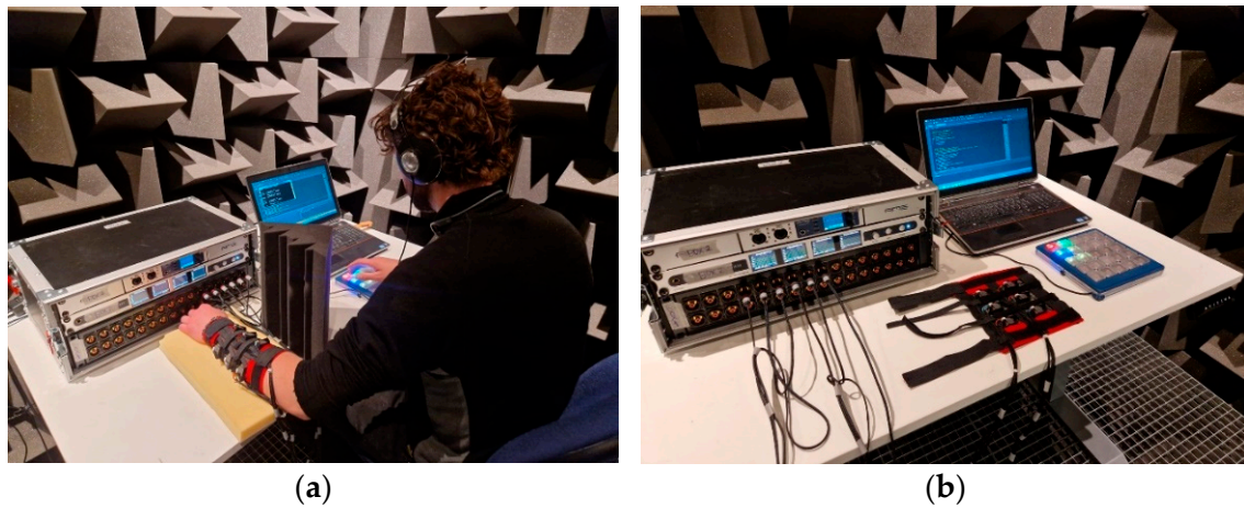
Figure 3. (a) A participant in the anechoic chamber wearing a vibrotactile sleeve, with his hand resting on a cushion. The participants wore headphones playing white noise to block out external auditory cues and responded to the vibrotactile feedback by pressing the correct keys on the keypad. (b) The audio hardware consisted of a digital audio interface (RME MADI face XT), digital-to-analog converters (Ferrofish A32), multi-channel amplifiers, and parallel vibrating voice coil actuators (Lofelt L5), t L5). The MADI face XT receives information from a computer via a USB cable and sends the signal to the Ferrofish A32 Analog-to-Digital/Digital-to-Analog (AD/DA) converter. Ferrofish A32 then conveys the signal to the amplifier, which then sends the amplified signal to the actuators.
